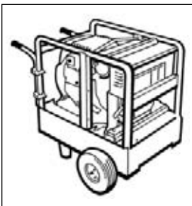
Stable Power* 110–125 volts, 60 Hz *Use 5,000 watt (min.) generator with one 20A GFCI protected circuit per tool. Two tools per 5,000 watt generator.
