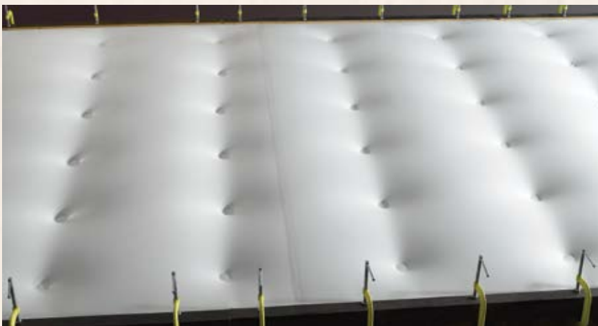
The RhinoBond welded membrane spreads the wind load evenly across the roof (above) as opposed to the traditional in-seam fastening method (below).
