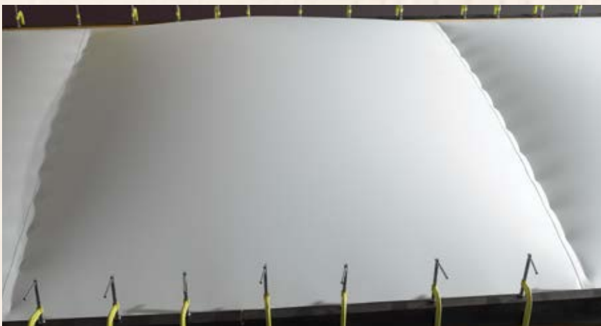
The RhinoBond welded membrane spreads the wind load evenly across the roof (above) as opposed to the traditional in-seam fastening method (below).
