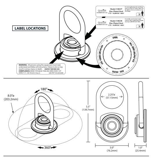
Tensile Strength (UTS): 10,000-lbf (44kN) Working load: 2,000-lbs (907kg) Weight: 1.2-lbs (544.3g) Materials: zinc plated steel Regulatory Compliance: Meets or exceeds ANSI Z359.1-2007, Z359.7-2011 and OSHA 1926.502 / EN 795:2012 Class A
