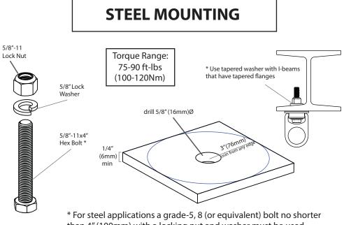
than 4" (100mm) with a locking nut and washer must be used. Swivel anchor must be flush with steel surface. A 16mm bolt may be used in place of a 5/8"-11 for metric applications.
